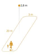
Possible mounting height: 2,50 m - 3,50 m Orange: radial and tangential
